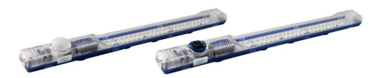
These lamps can be mounted to the panel either with clips (supplied) or by the magnets on the back. A strong connection is made by the spring-loaded terminal blocks (located at each end of the device, allowing daisy-chain assembly of up to 16 lamps in AC, up to 8 lamps in DC). Wire size must be 0.3-1.3 mm<sup>2</sup> (22-16AWG).
