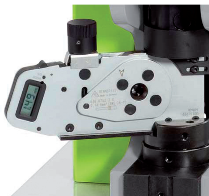
Digital indenter with incorporated positioner
