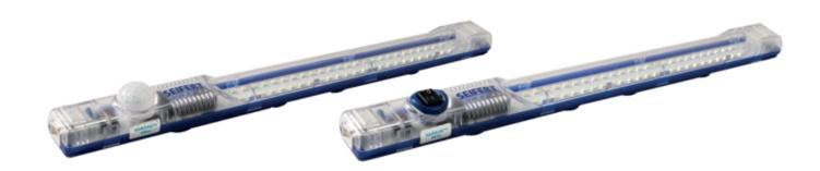
These lamps can be mounted to the panel either with clips (supplied) or by the magnets on the back. A strong connection is made by the spring-loaded terminal blocks (located at each end of the device, allowing daisy-chain assembly of up to 16 lamps in AC, up to 8 lamps in DC). Wire size must be 0.3-1.3 mm<sup>2</sup> (22-16AWG).
