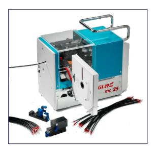
The MC 25 is a portable electric machine that applies, **ferrules in strip** form from 0.5 mm<sup>2</sup> (22AWG) to 2.5mm<sup>2</sup> (14AWG) onto unprepared insulated stranded wires.
